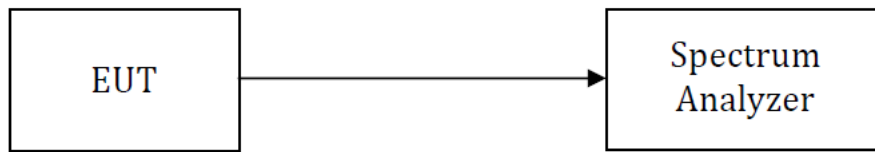
Test Setup Block Diagram
