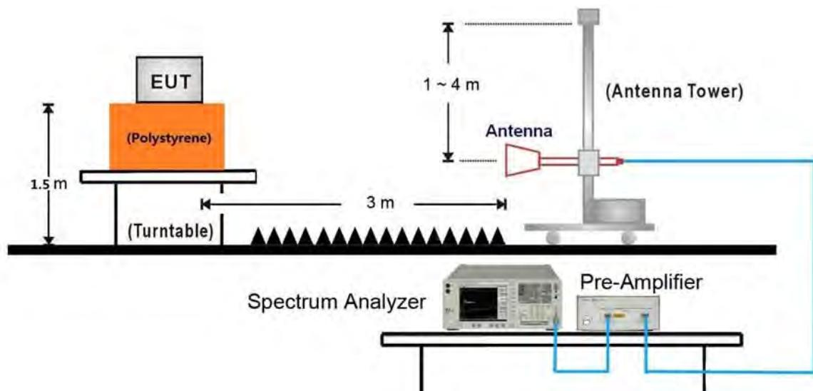
18GHz ~25GHz Test Setup:
