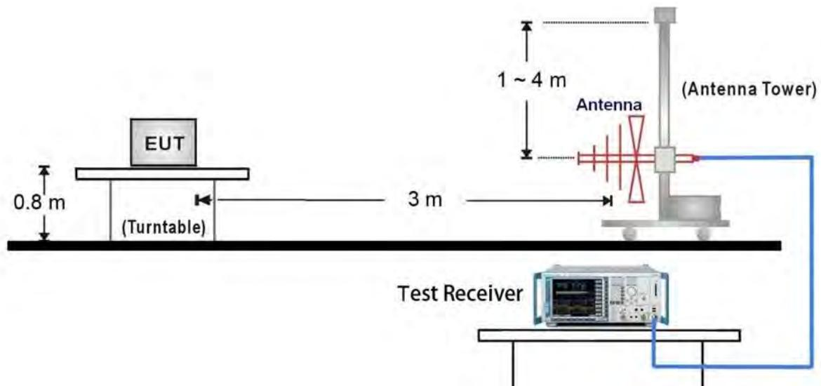
1GHz ~ 18GHz Test Setup:
