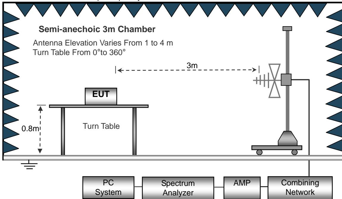
(C) Radiated Emission Test-Up Frequency Above 1GHz
