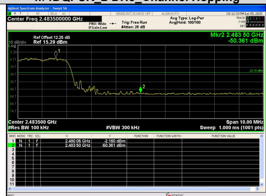
Out Of Band Emission(Right) \pi/4 DQPSK_2-DH5_Channel Hopping
