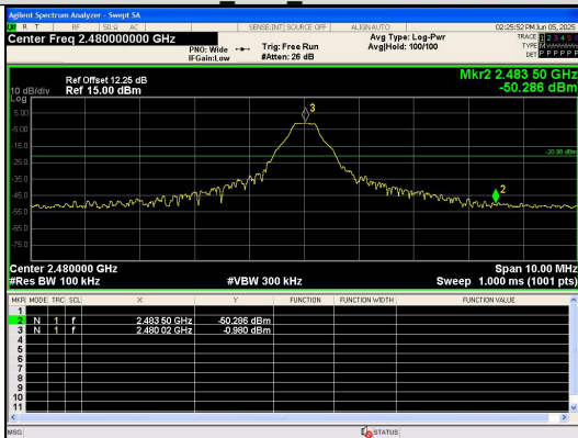
Out Of Band Emission GFSK_DH5_Channel 78
