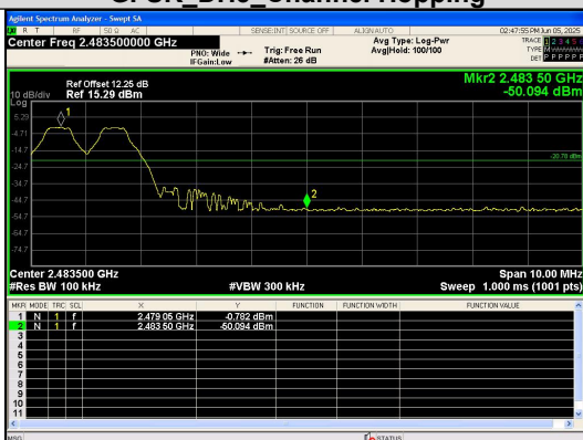
Out Of Band Emission(Right) GFSK_DH5_Channel Hopping
