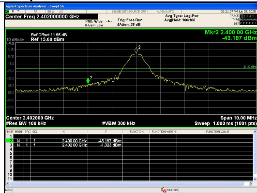
Out Of Band Emission GFSK DH5 Channel 0
