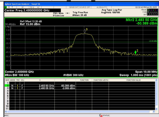
Out Of Band Emission \pi/4 DQPSK_2-DH5_Channel 78
