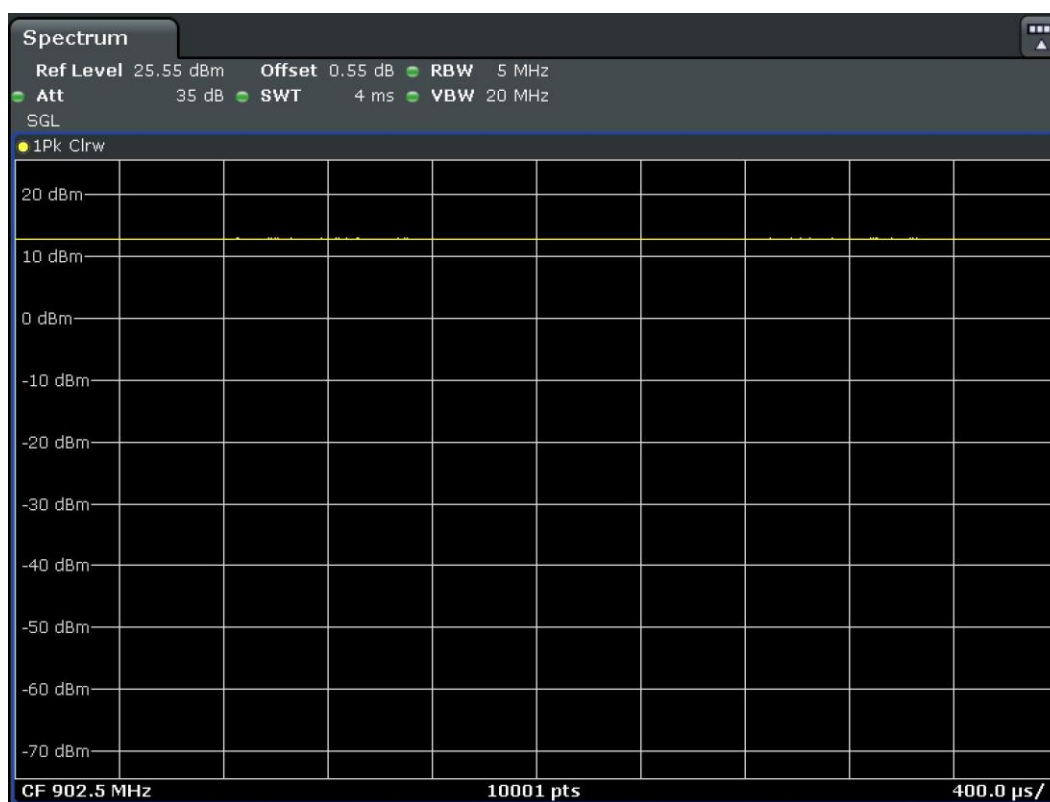
Figure 1. Antenna-Port Conducted Measurements, Duty Cycle: Low Channel, 902.5 MHz Plot
