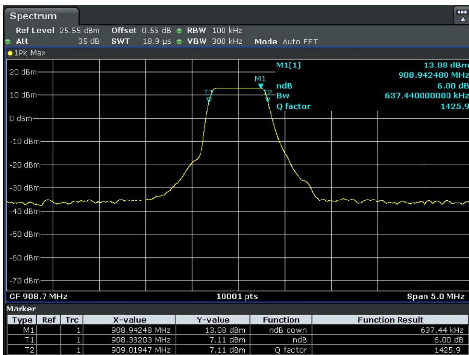
Figure 3. Antenna-Port Conducted Measurements, 6dB DTS Bandwidth: Mid Channel, 908.7 MHz Plot
