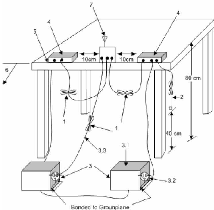
1—Interconnecting cables that hang closer than 40 cm to the ground plane shall be folded back and forth in the center forming a bundle 30 cm to 40 cm long.
