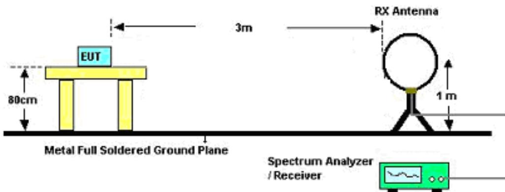
Magnetic field tests shall be performed in the frequency range of 9 kHz to 30 MHz using a calibrated loop antenna. The center of the loop shall be 1 m above the ground.
