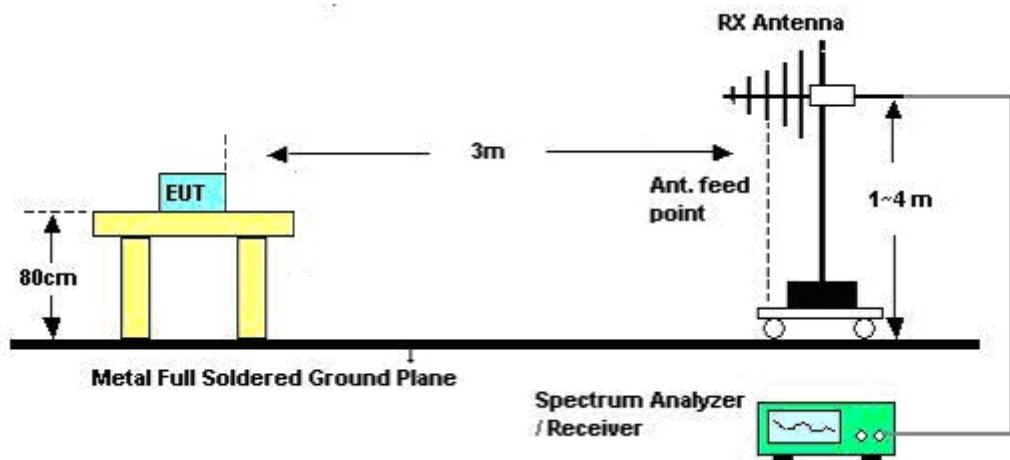
Electric field tests shall be performed in the frequency range of 30 MHz to 1000 MHz using a calibrated bi-log antenna. the antenna height shall be varied from 1 m to 4 m.
