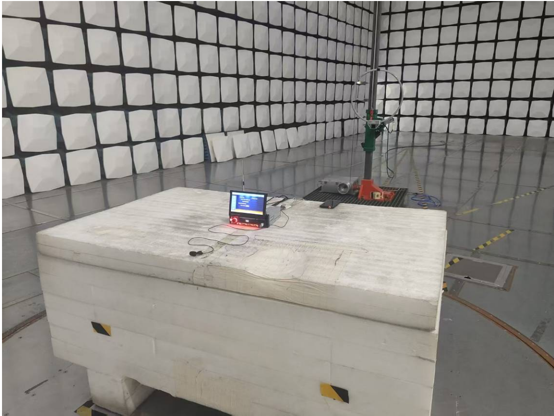
Radiated Emission 9kHz-30MHz Perpendicular View
