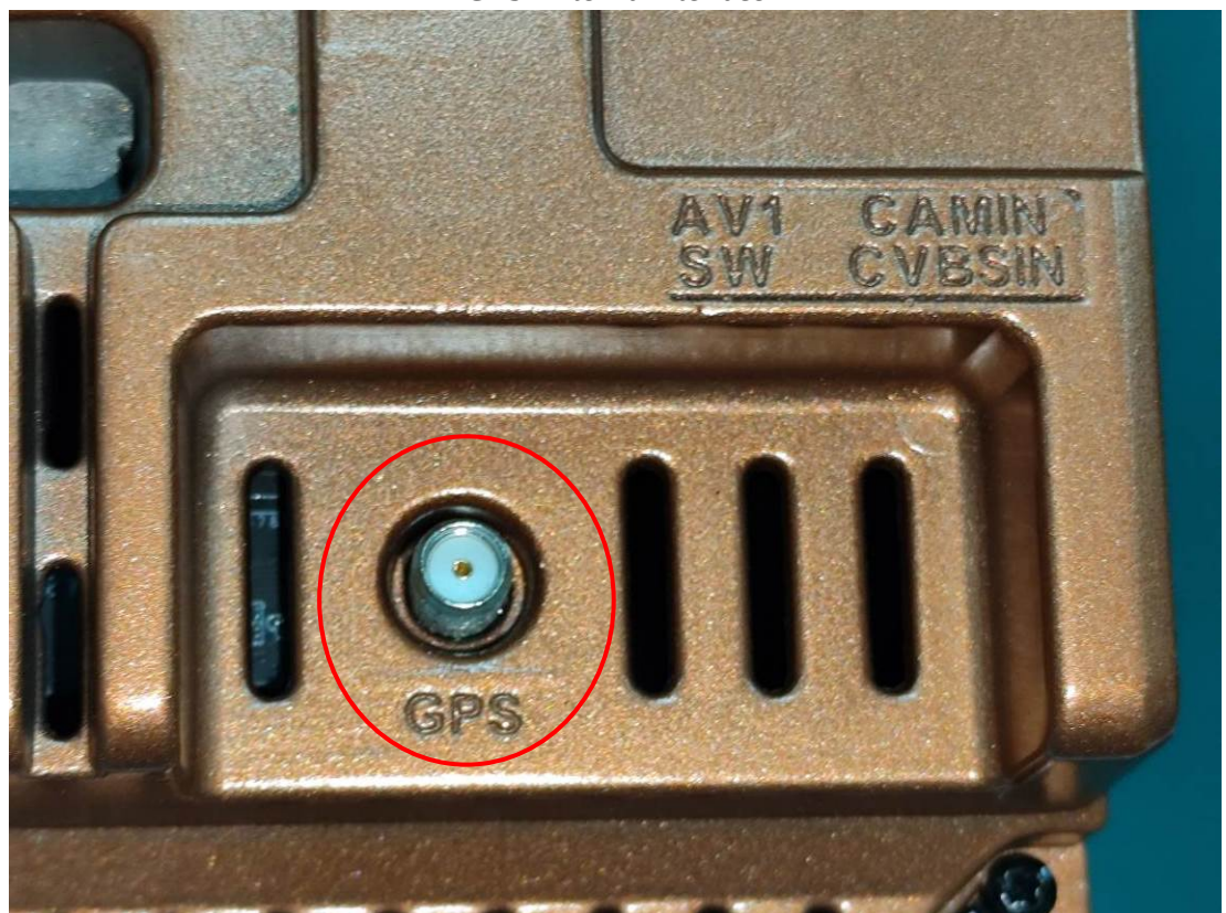
GPS Antenna Interface
