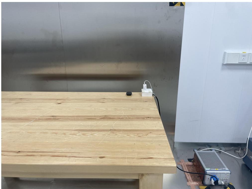
Radiated Emission Test View|(Below 1G)
