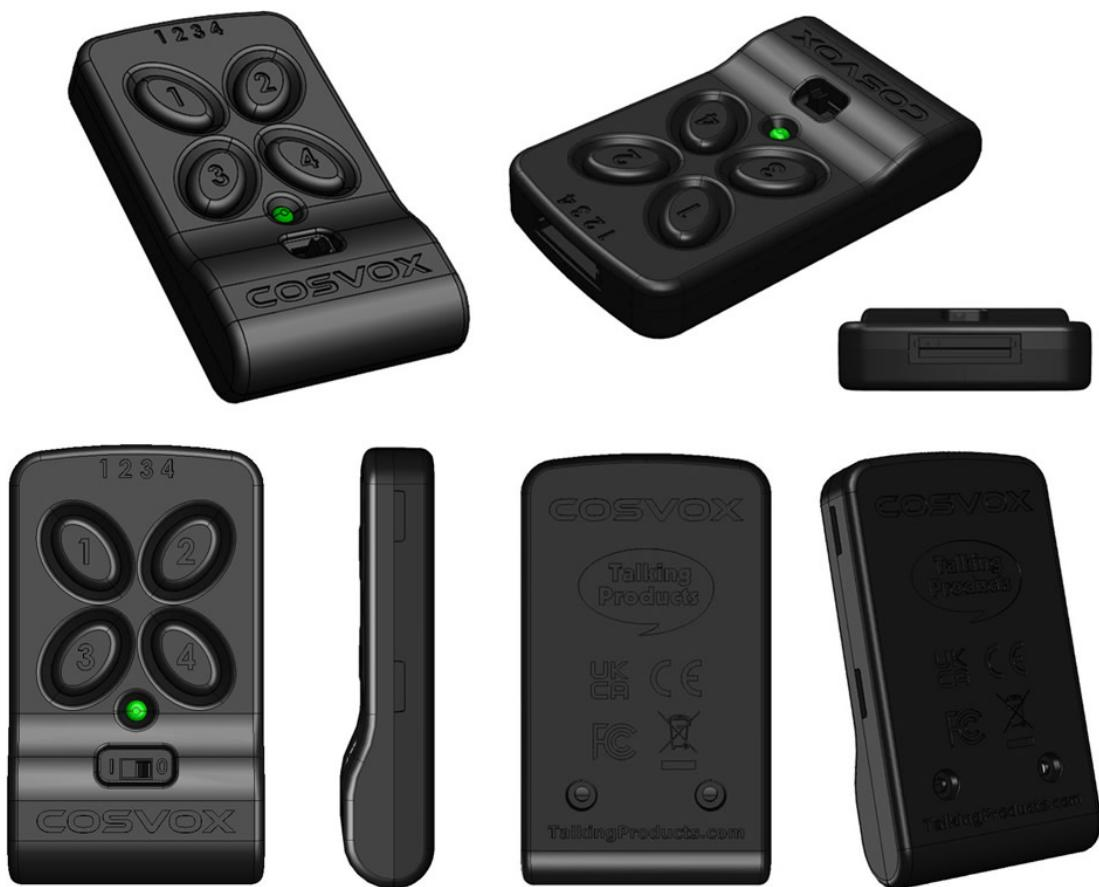
2a) The key fob has 4 buttons on the front. There must be Bluetooth connection between the Sound Module and the Key Fob.
