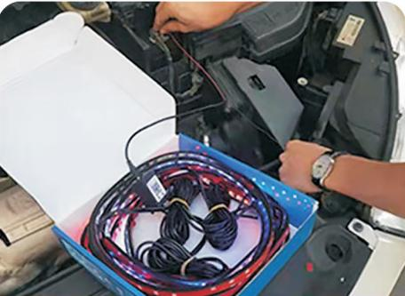
Always test the lamp before installation. (try 12 volt power)
