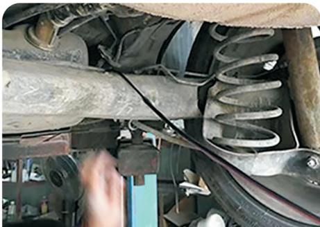
Fix the cable passing through the tire in the inactive position with the cable flange.
