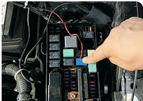
Connect the fuse box to the ACC power supply or the headlamp fog lamp
