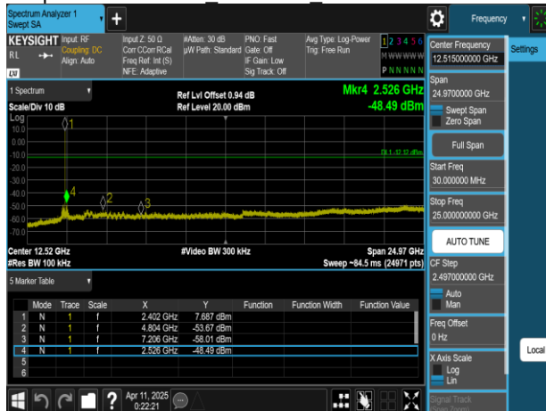
Spurious Emission BLE 125k MidCH20-2442MHz
