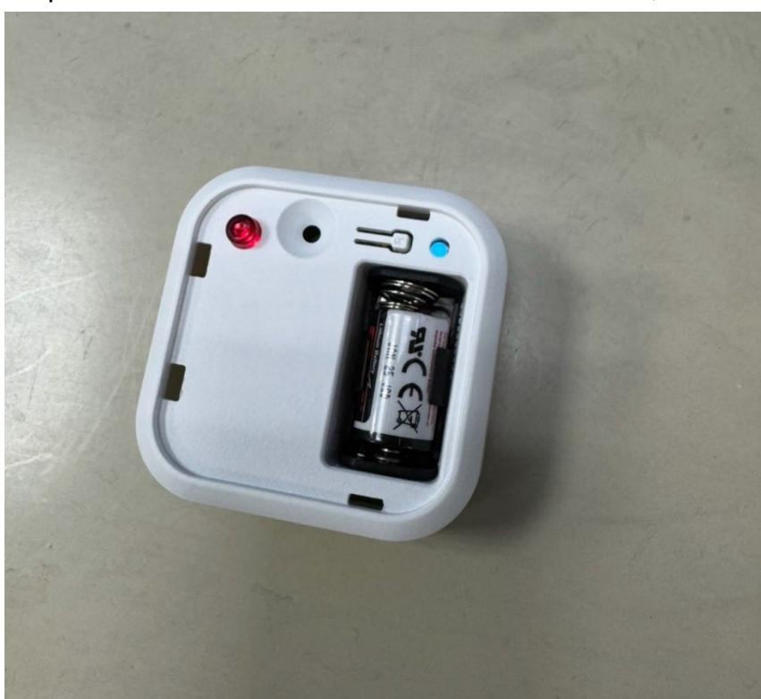
Step 3 : To learn the signal, direct the remote control to the side of the TARUIE AC REMOTE. Then, press the power button on the remote control. The learning process is successful when the blue light turns off.
