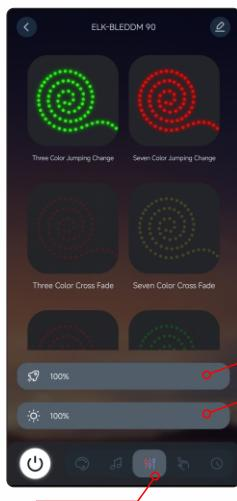
Speed slider to control the speed of dynamic mode.
