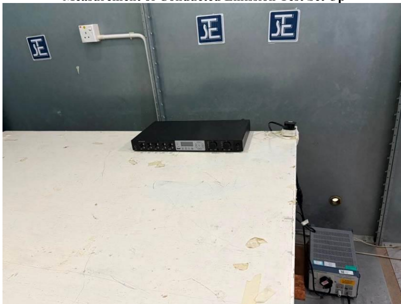
Measurement of Conducted Emission Test Set Up
