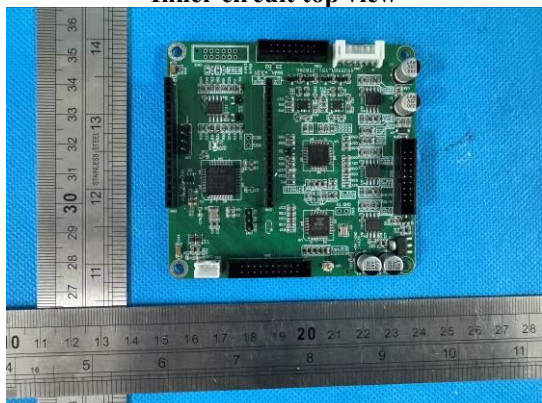
Inner circuit top view
