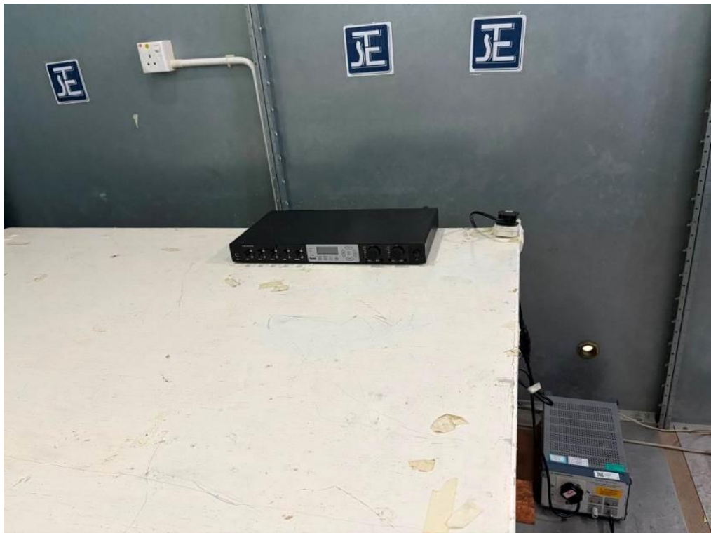
Measurement of Conducted Emission Test Set Up
