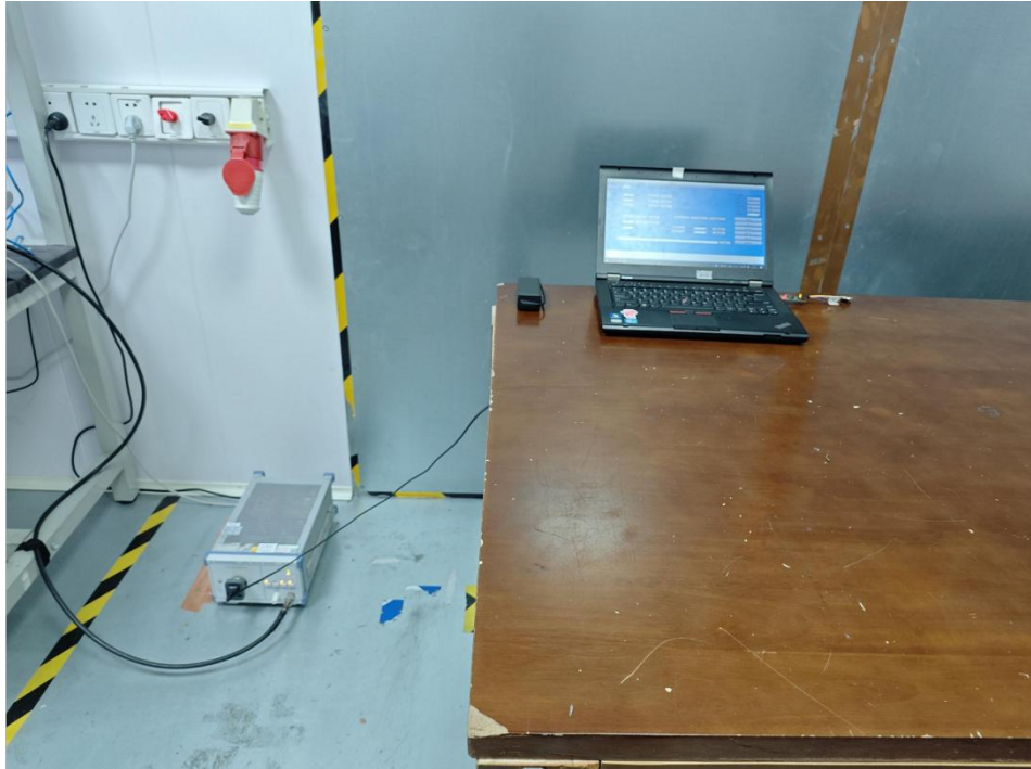
Conducted emissions at AC power line (150kHz-30MHz)
