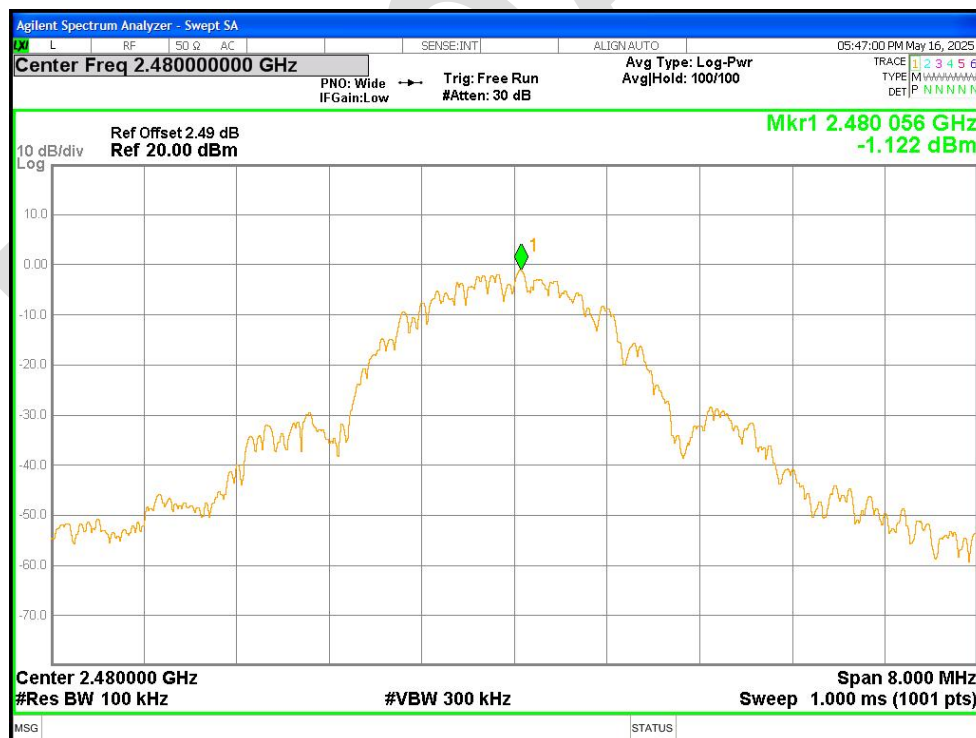
Band Edge NVNT ZIGBEE 2480MHz Ant1 Ref
