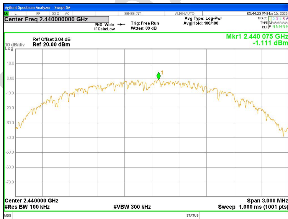
Tx. Spurious NVNT ZIGBEE 2440MHz Ant1 Emission
