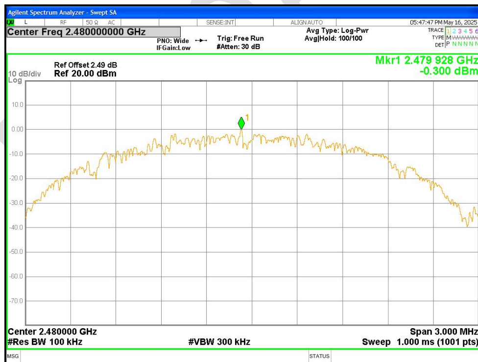
Tx. Spurious NVNT ZIGBEE 2480MHz Ant1 Ref
