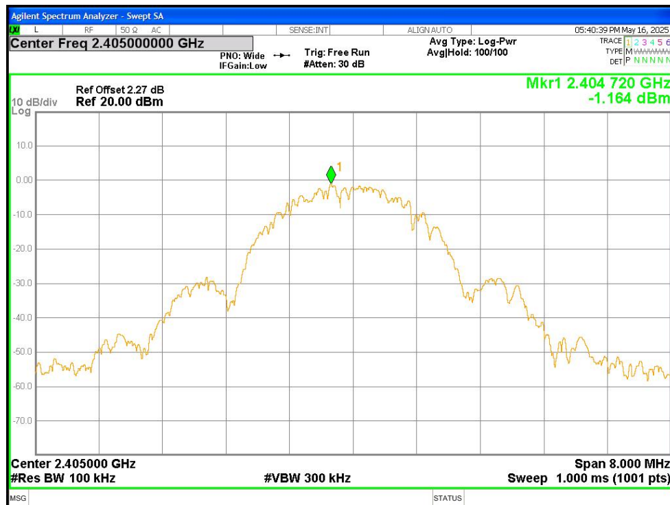
Band Edge NVNT ZIGBEE 2405MHz Ant1 Emission
