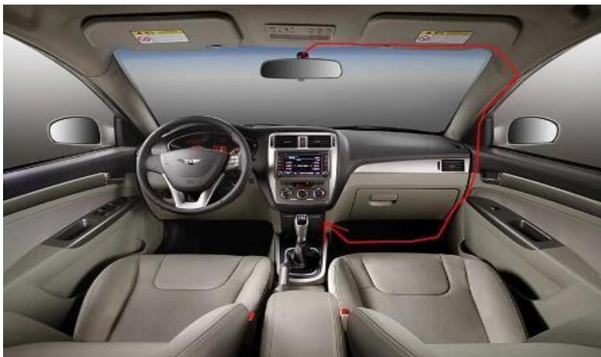
**Note:** When wiring, the extension cord of the vehicle charger can be hidden and installed along the top trim panel of the automobile windshield, as shown in the above figure.
