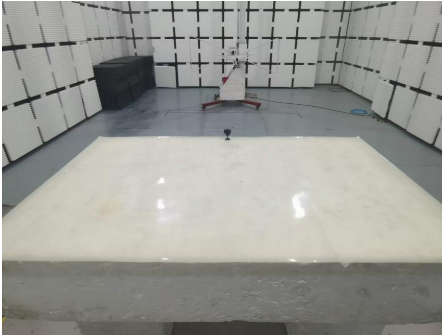
Set-up for Radiated Spurious Emission, Above 1GHz
