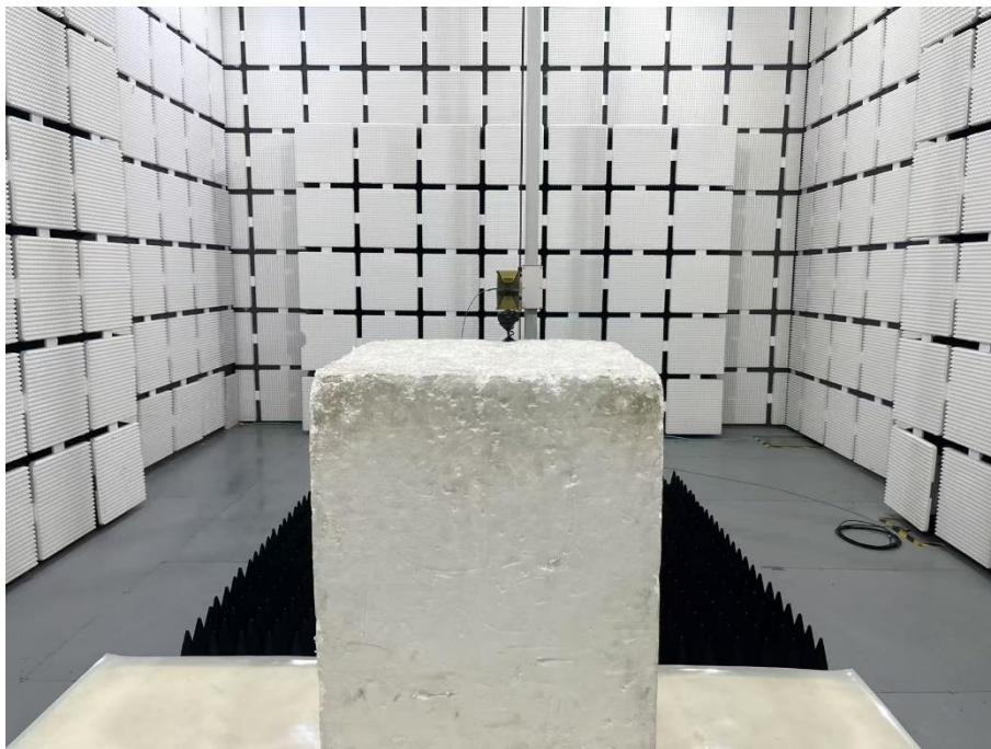
Set-up for Radiated Spurious Emission, Above 1GHz
