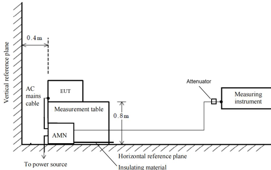
Note: the distance between LISN and Vertical reference plane is 40 cm and the distance between LISN and EUT is 80 cm.
