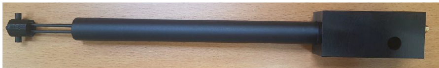
Figure 1 – MVG COMOSAR Validation Dipole
