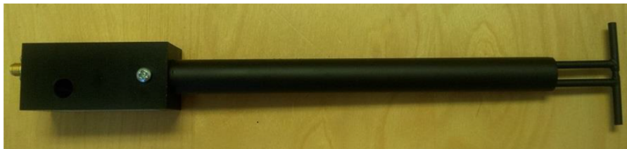
Figure 1 – MVG COMOSAR Validation Dipole
