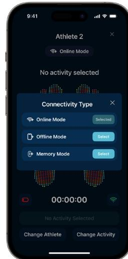
5.3.3. By pressing the battery icon to the left of the timer, you can view the battery level of the pods.
