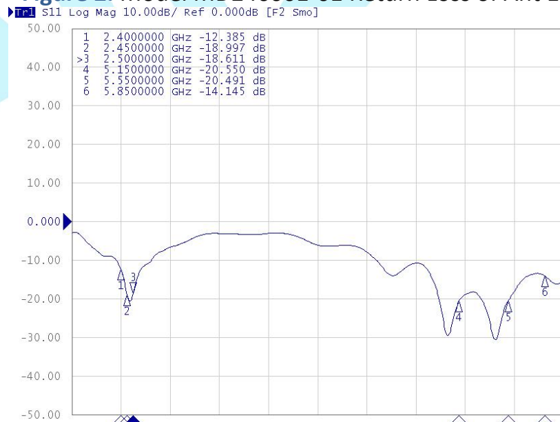
Figure 3: Model MD246001-01 Return Loss of Ant 2
