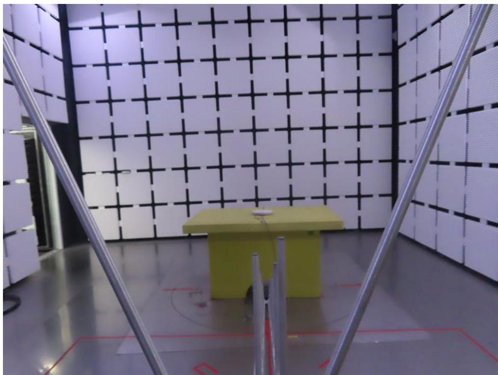
**Radiated Emissions Test Photos****Band edge & Harmonic(1 GHz to 18 GHz)**
