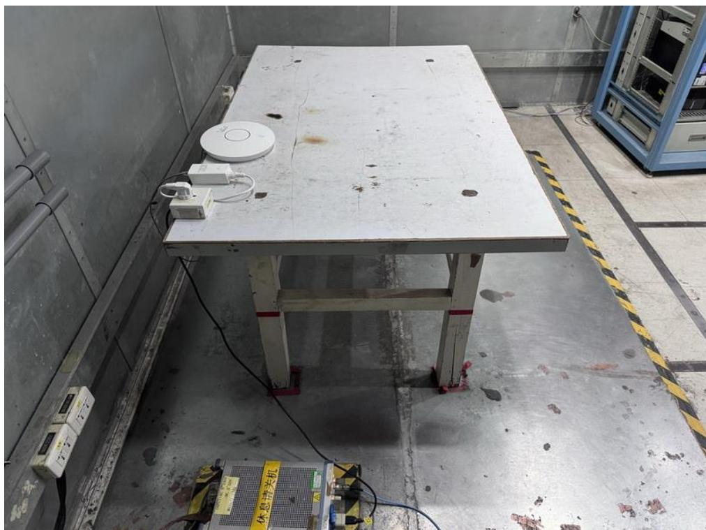
**Radiated Emissions Test Photos****9 kHz to 30 MHz**
