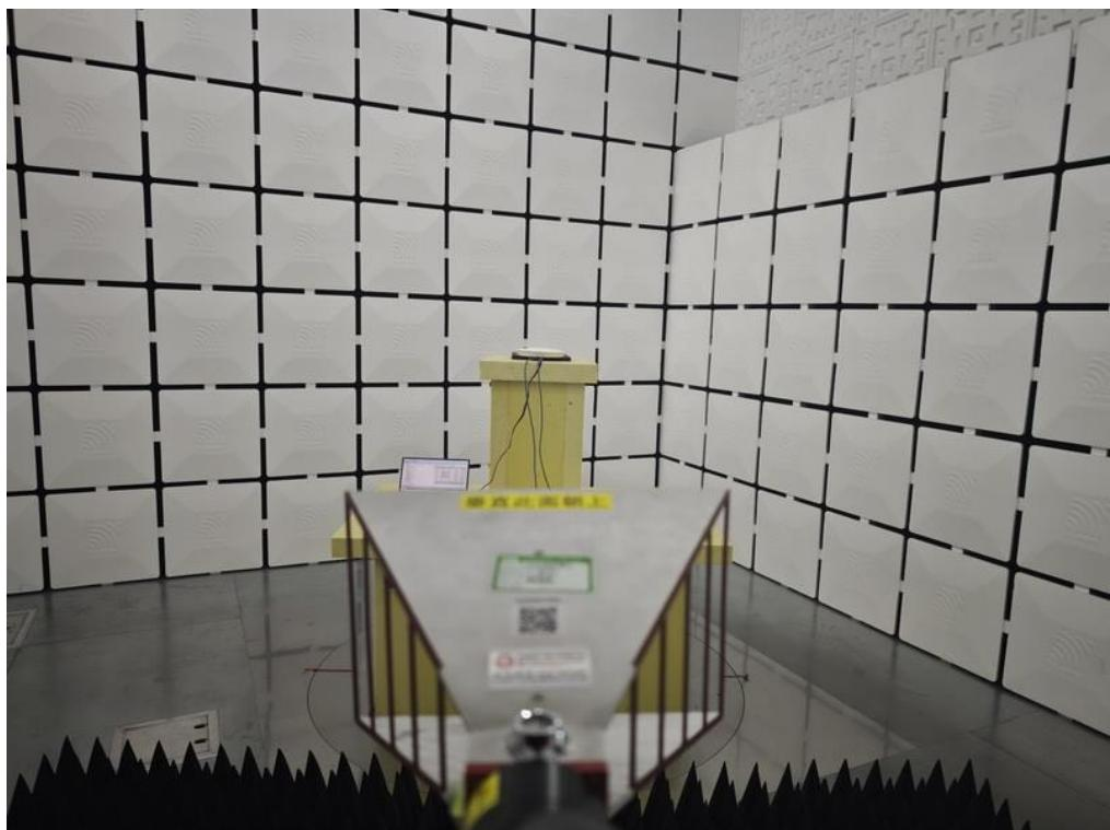
**Radiated Emissions Test Photos****Harmonic(18 GHz to 26.5 GHz)**
