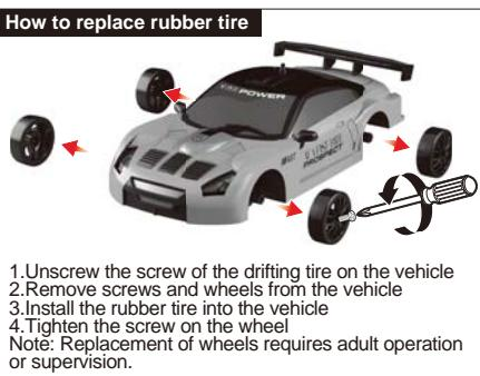
1. Unscrew the screw of the drifting tire on the vehicle
