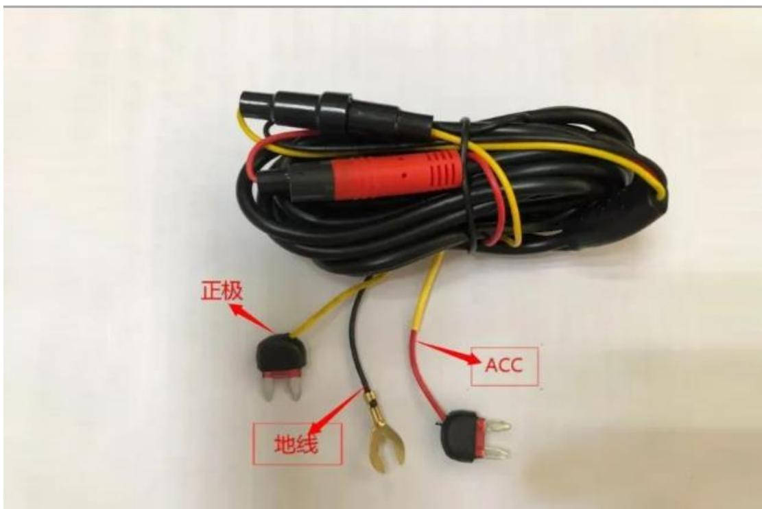
1. As shown in the figure above: Connect the yellow power cord to the 12V power supply, the red ACC ignition control line, the black ground, start the car engine, and see the blue light on and flashing. The machine starts and enters the automatic recording state.
