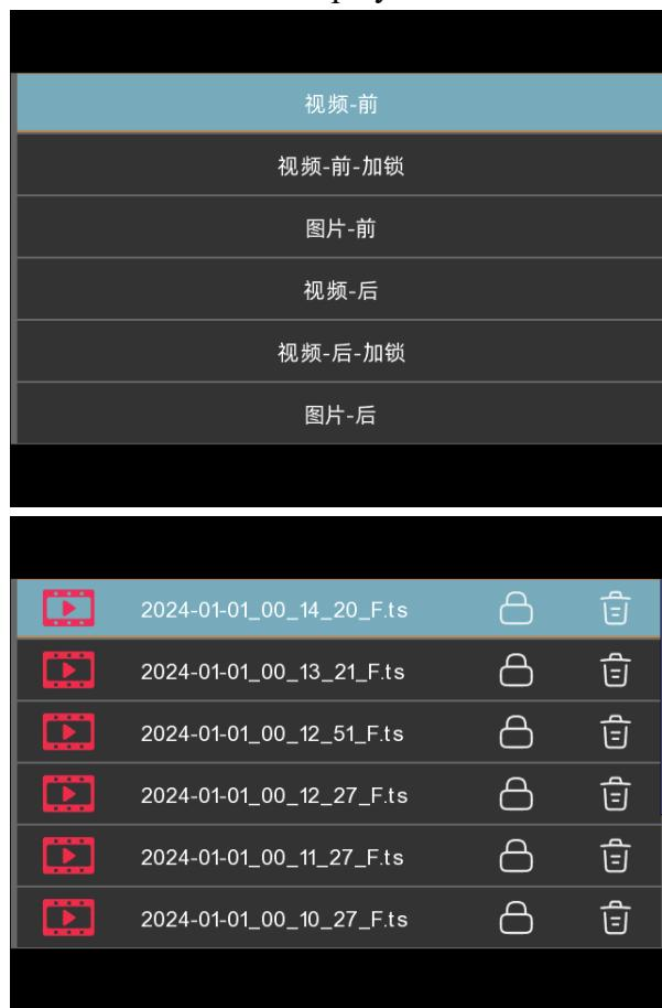
Short press the up button to select the file, short press the down button to select the file, short press the OK button to play, short press the menu button to return to the previous level; short press the lock button to add/unlock files in the list interface (no function in the picture file list), short press the M button to delete files; short press the OK button to pause/start playing when playing files, short press the up/down button to switch file playback
