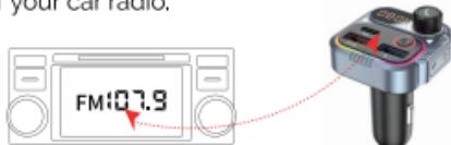
5. FM transmitter frequency setting: Press until the frequency display flickering, rotate button to adjust the transmitter's frequency to be the same as the frequency on the car radio.
