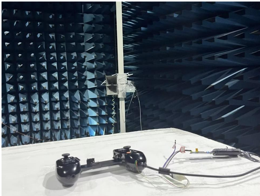
Radiated Spurious Emissions Above 1GHz
