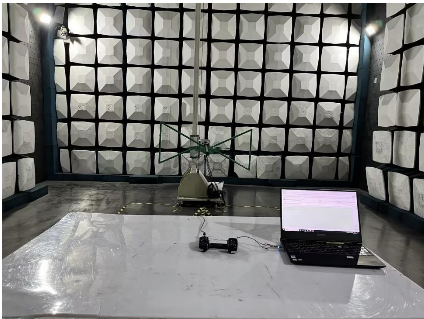
Radiated Spurious Emissions Below 1GHz
