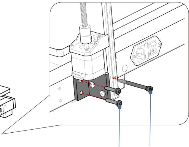
\*It is recommended to use allen key with short sides to secure the screws.
