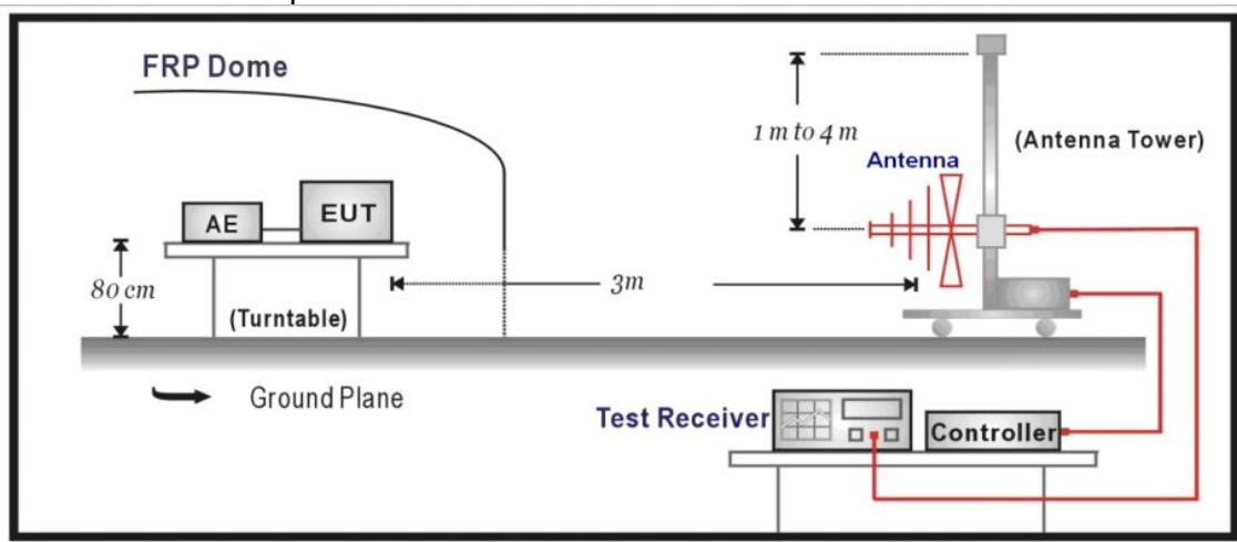
1GHz -40GHz Test Setup:
