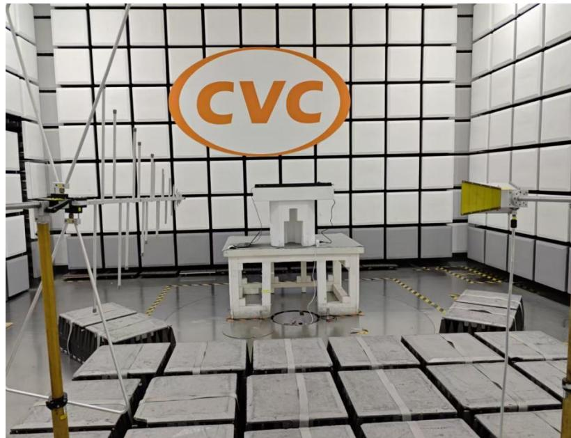
Description: Radiation test photo(frequency range: 18GHz-40GHz)
