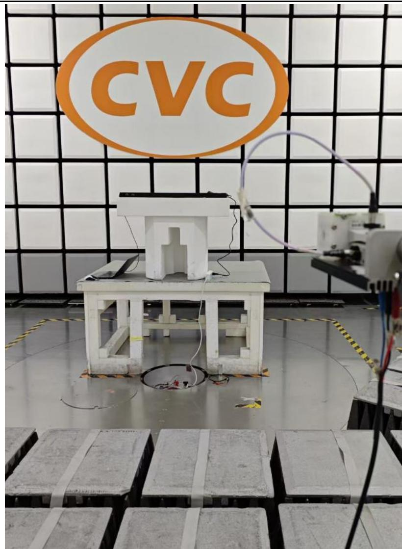
Description: Radiation test photo(frequency range: 30MHz-1GHz)
