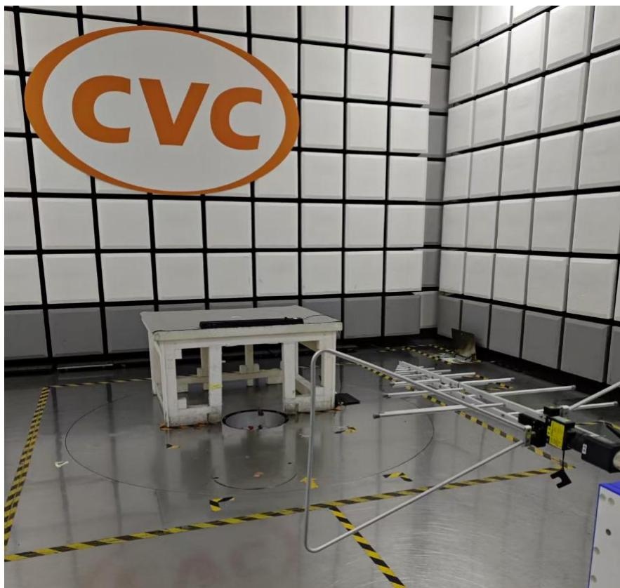
Description: Radiation test photo(frequency range: 9kHz-30MHz)
