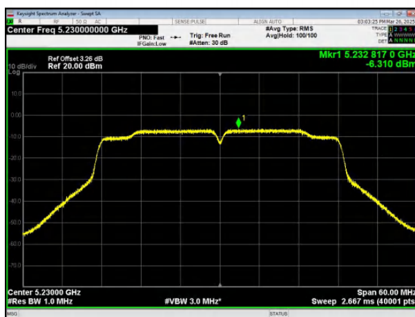
(802.11ac40) PSD plot on channel 46
