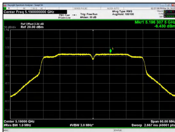
(802.11n40) PSD plot on channel 46
