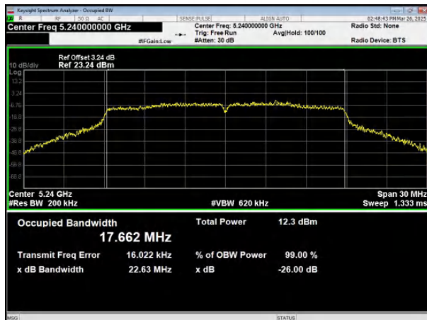
(802.11 n20) 26dB Bandwidth plot on channel 48
