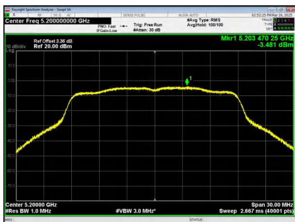
(802.11ac20) PSD plot on channel 40
