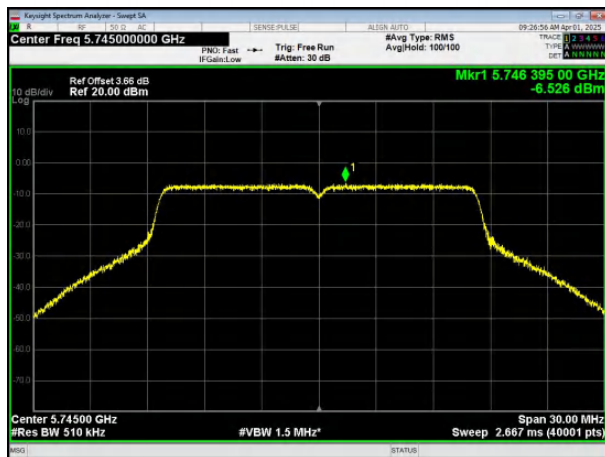
(802.11a) PSD plot on channel 157
