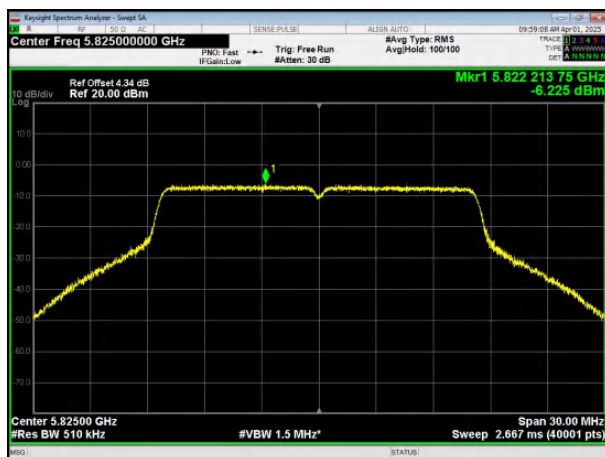
(802.11a) PSD plot on channel 165
