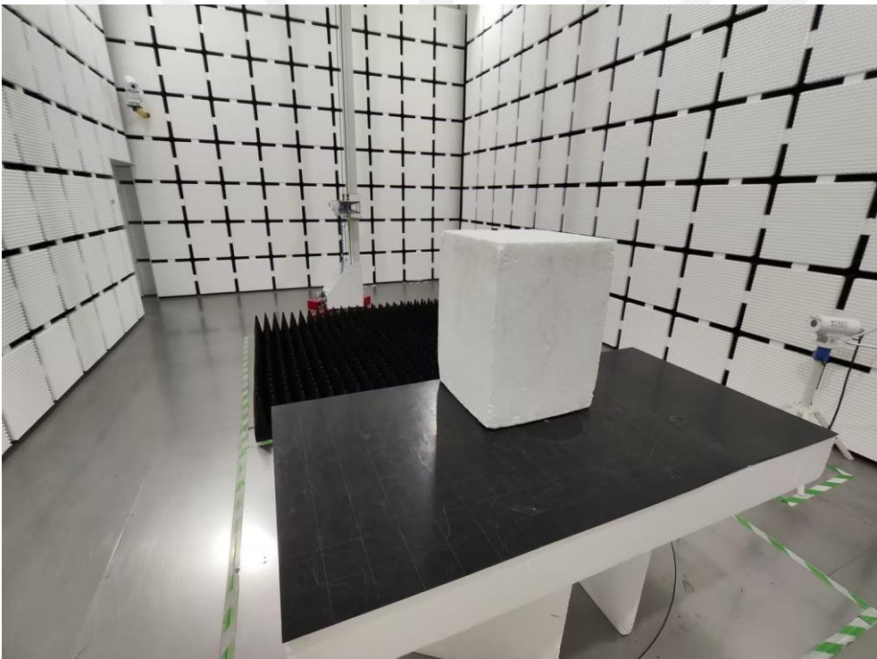
Spurious Radiation Emissions Test (<1G)
