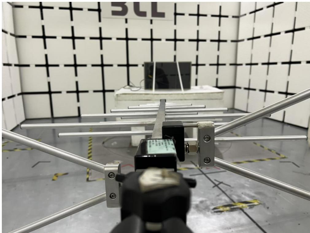
**Radiated Emissions Test Photos****Above 1 GHz**
