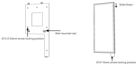
1. After confirming the installation position, fix the wall hanging securely. The installation position should be less than 2 meters from the ground. (Can be locked with ST3.5 \* 25mm screws for wall mounting)
