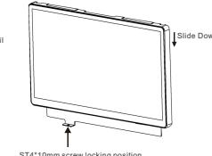
1. After confirming the installation position, fix the wall hanging securely. The installation position should be less than 2 meters from the ground. (Can be locked with ST3.5 \* 25mm screws for wall mounting)
