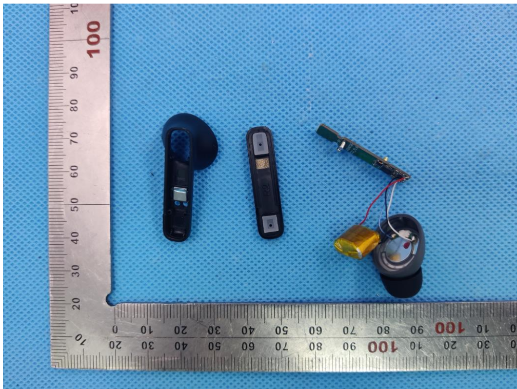
Open view-1 of EUT(Right Ear.)
