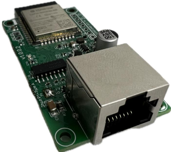
The BLE Dongle is made appositely to be connected to Audio Enhancement's classroom amplifiers or control solutions via the RJ45 "Remote Port". The pin-out of the BLE Dongle RJ45 connection is as follow:
