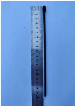
The total length of the antenna is 205MM
