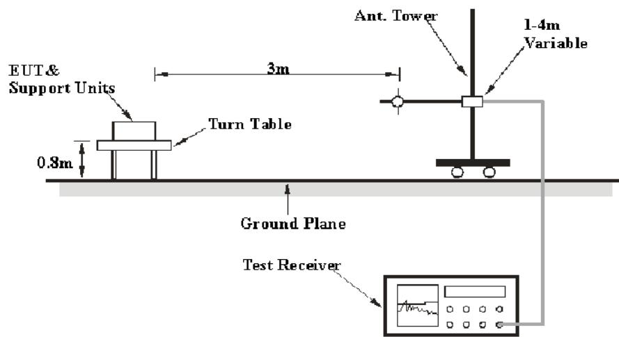
The radiated emission tests were performed in the 3-meter chamber a test site, using the setup accordance with the ANSI C63.10-2020.
