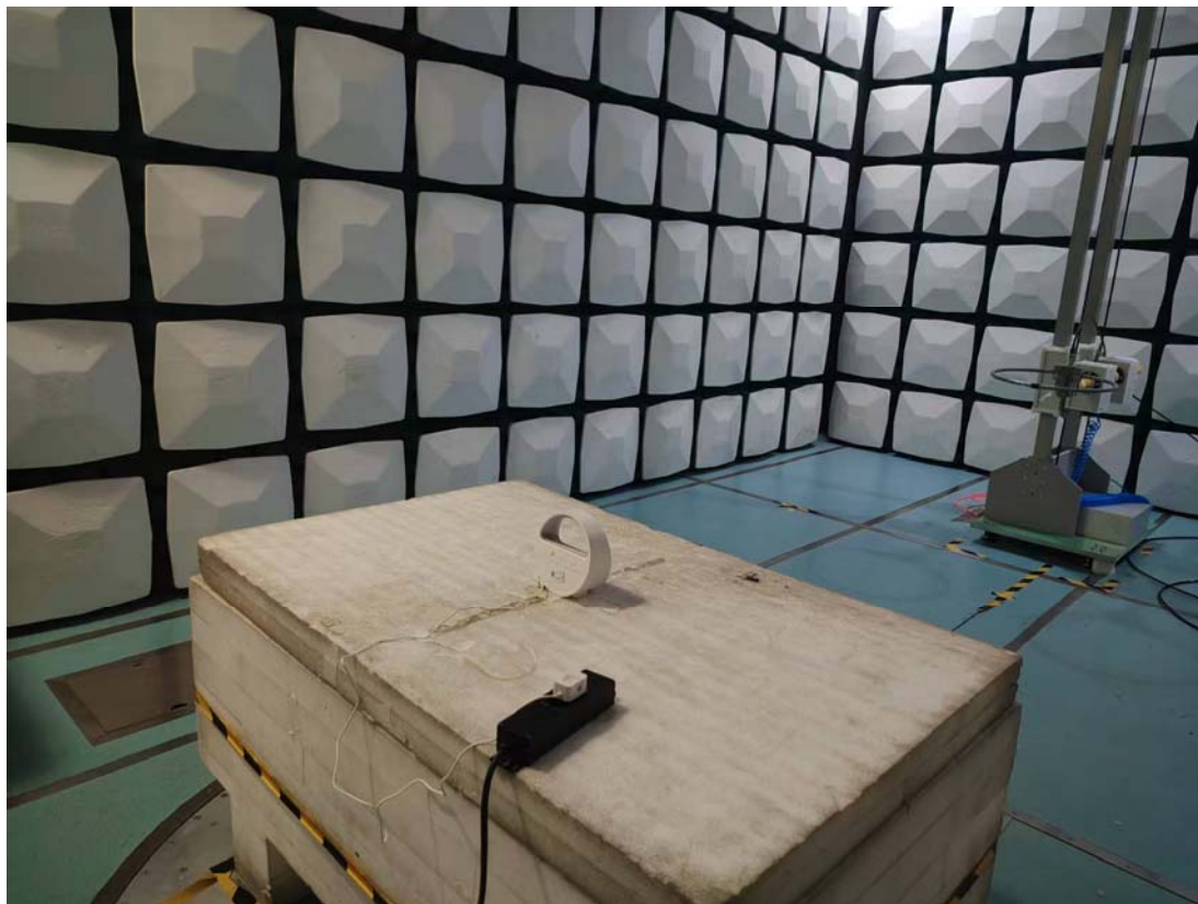
Radiated Emission 30MHz-1GHz View
