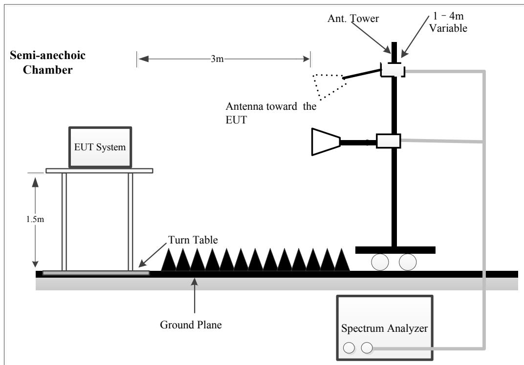
The radiated emissions were performed in the 3 meters distance, using the setup accordance with the ANSI C63.10-2020. The specification used was the FCC 15.209, and FCC 15.247 limits.
