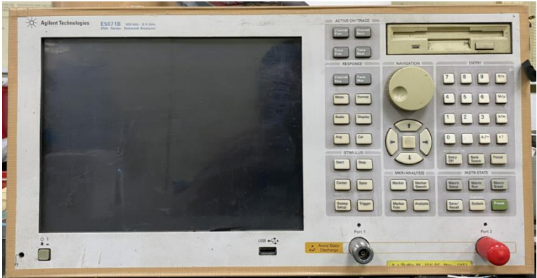
Agilent 5071B (S Parameter (RL/VSWR) Test Equipment)
