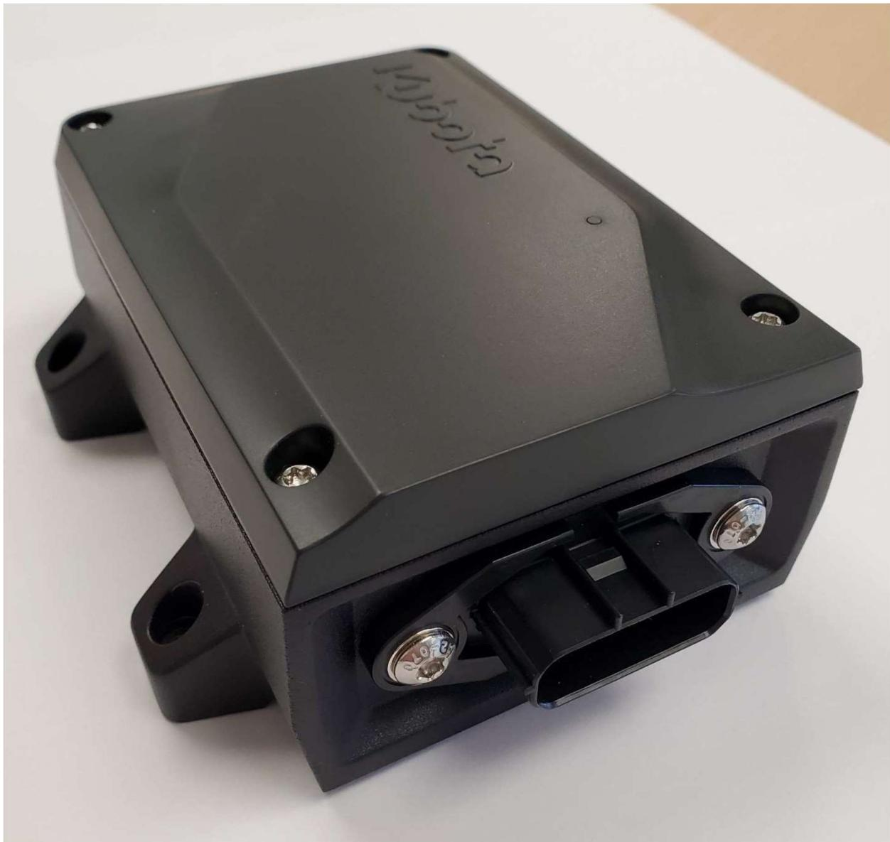
The ECU image shows the IP67 water and dust proof enclosure, the external 24 pin connector, the composite cover with the Kubota logo and power/fault indicator, and the aluminum powder coated base.
