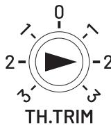
Turn the knob clockwise and the car will cruise forward. The larger the number, the faster the speed.
