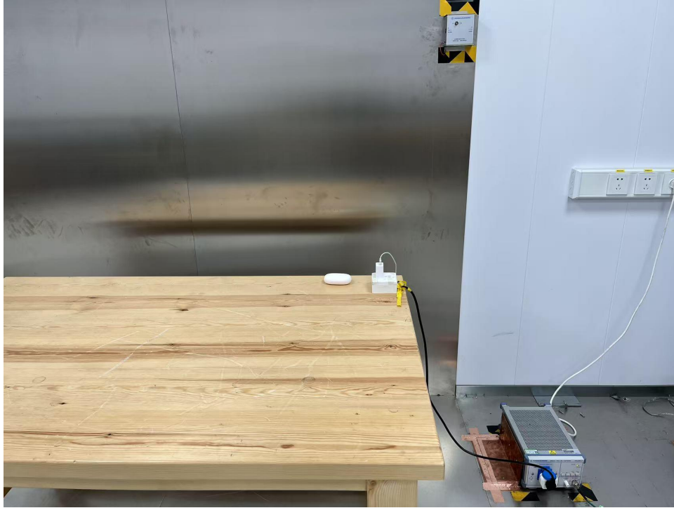
Radiated Emission Test View|(Below 1G)
