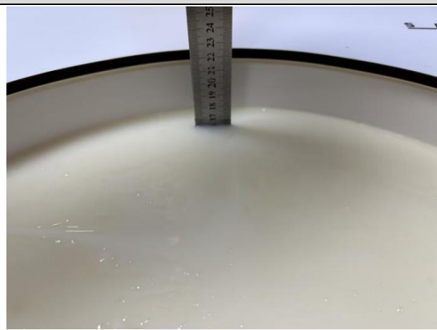
Photo 1: Tissue Simulant Liquid for Head 700- 3000MHz
