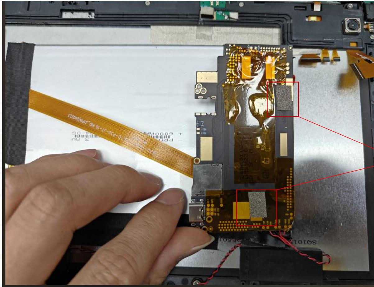
5: Conductive wool is attached to the back of the motherboard and grounded to the screen
